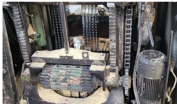
Fig. 1. Sawmill no. 1 with the visible 30 kW motor on the right side, driving the set of vertical saws. [Own work]
