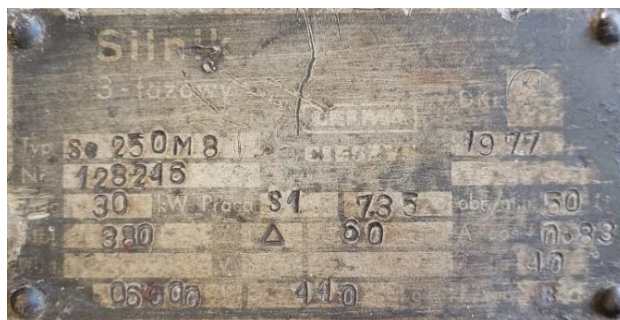
Fig. 2. Nameplate of a 3-phase 30 kW motor. [Own work]
