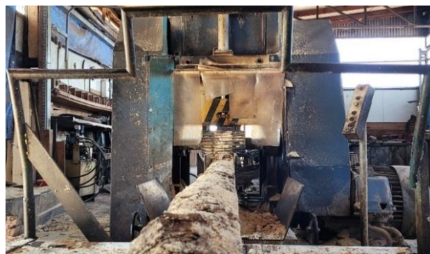
Fig. 3. The sawmill no. 1 with the motor (5 kW) visible on the right, driving the log feeder unit. [own work]
