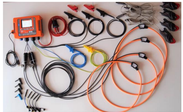
Fig. 8. SONEL PQM-710 portable electricity analyzer with accessories. [own work]
